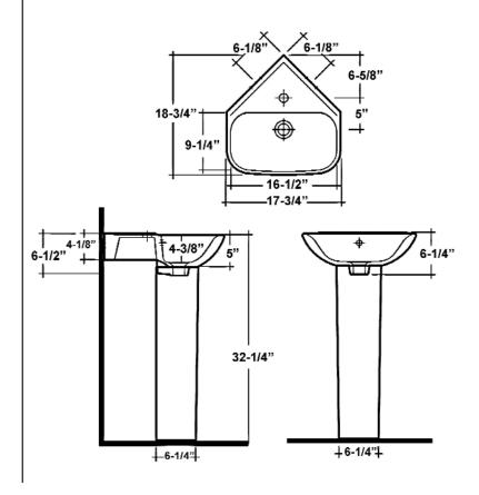
Dimensions of fixture are nominal and may vary within the range of tolerances established by ASME Standard A112.19.2-2018. Dimensions and specifications subject to change without notice.
